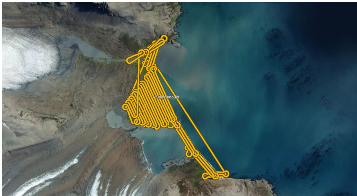
Figure 2. Flight path from the survey of St Andrews Bay which captured both the elephant seal and king penguin colony's. This flight was possible due to BVLOS permissions, taking a total of 56 minutes during which the eBee X flew 42.8 km.
